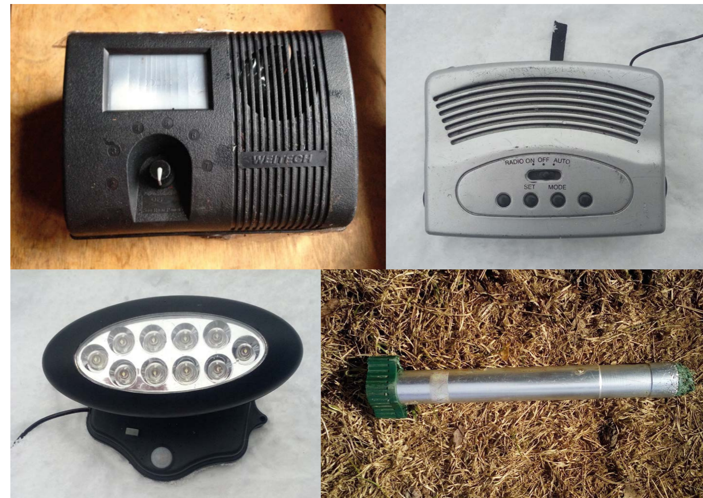
Fig. 1. Commercially available electronic devices tested for their influence on the behaviour of captive wolves: Weitech WK0051 Garden Protector (top left), radio (top right), motion-activated white light (bottom left) and Defenders mega-sonic mole repeller (bottom right).
