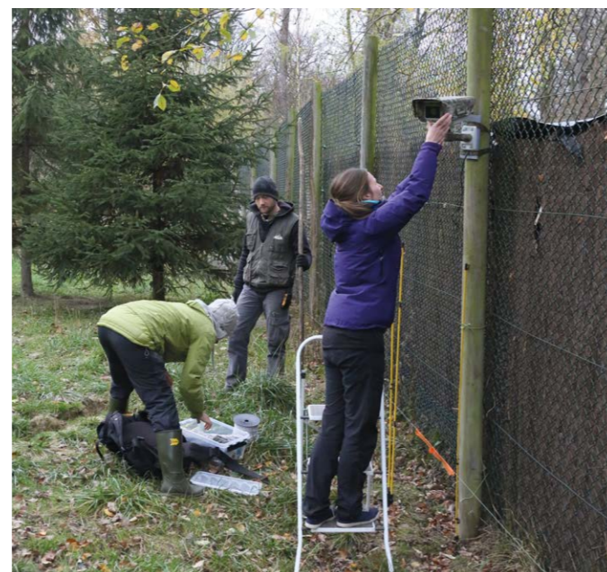
Fig. 2. Installation of the camera equipment: remote camera (Bushnell, above) and thermal camera (AXIS Q1921-E, below).
